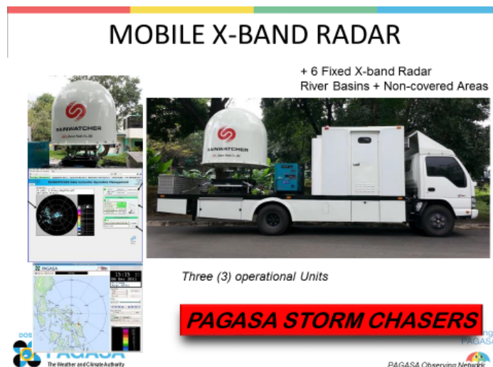
Figure G. A photo of the mobile X-band Radar used by storm chasers.
